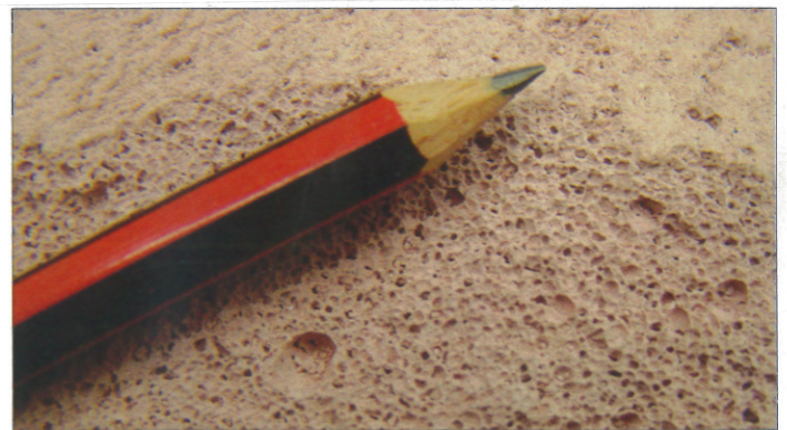
This photo shows the bubble like texture of the Hebel™ concrete panel.
