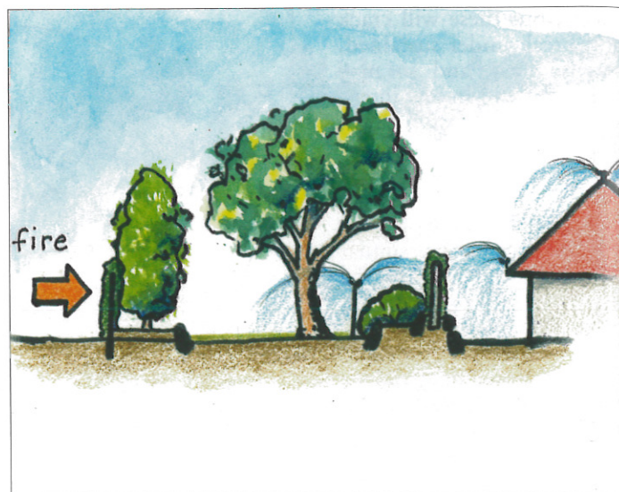
A possible set-up of multiple shields protecting a house in an ember attack with the added protection of a sprinkler system.
